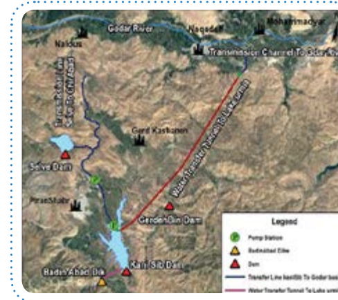
Water Transmission Tunnel Delivering the Surplus of the Gelas River to the Lake Urmia Basin
